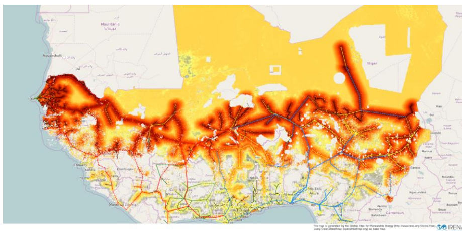
Figure 12: Suitability analysis for West Africa. Suitability scores for grid-connected solar power, not further than 75 km from the nearest grid. A suitability analysis looks at resource potential, distance to grid infrastructure, population density, topography, land cover and protected areas and ranks technical suitability to develop a project, ranked between 0 and
