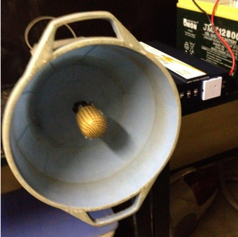
Figure 11: Coconut grating mill installed at Malahang - inverter and battery shown at right
