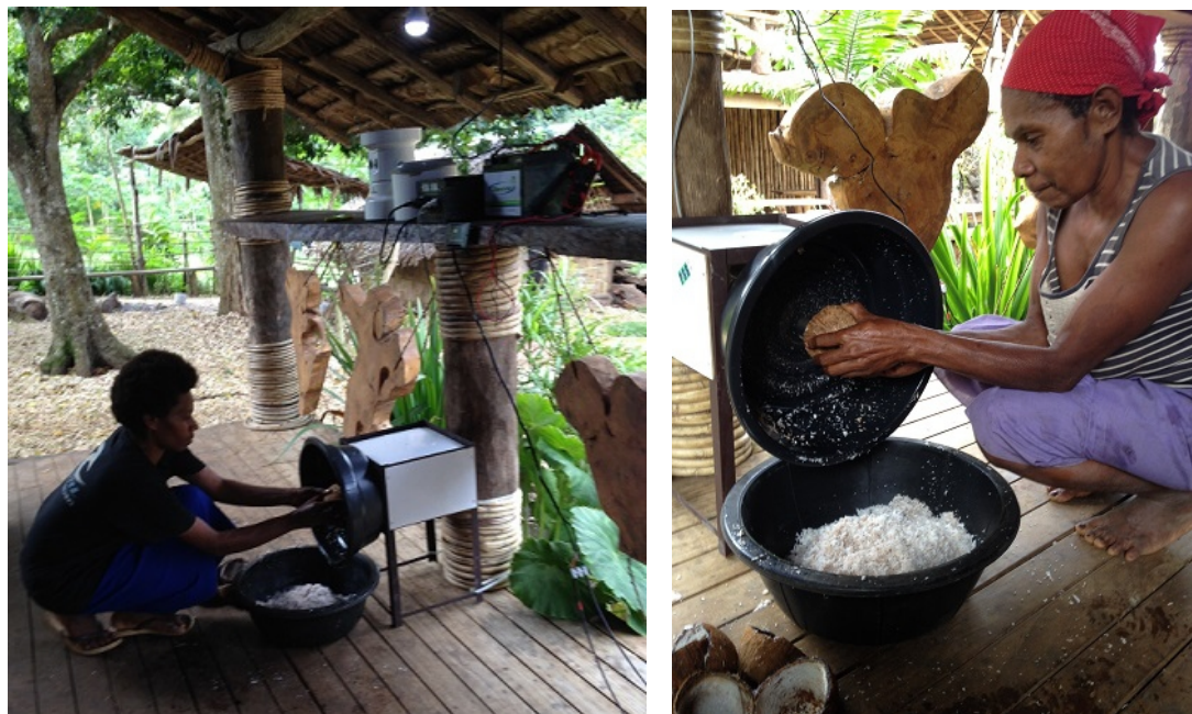
Figure 9: Coconut grating mill and Wondermill grinder set up with battery and inverter
