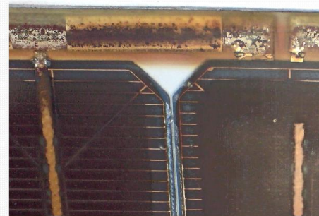
Corroded panel in Maldives
