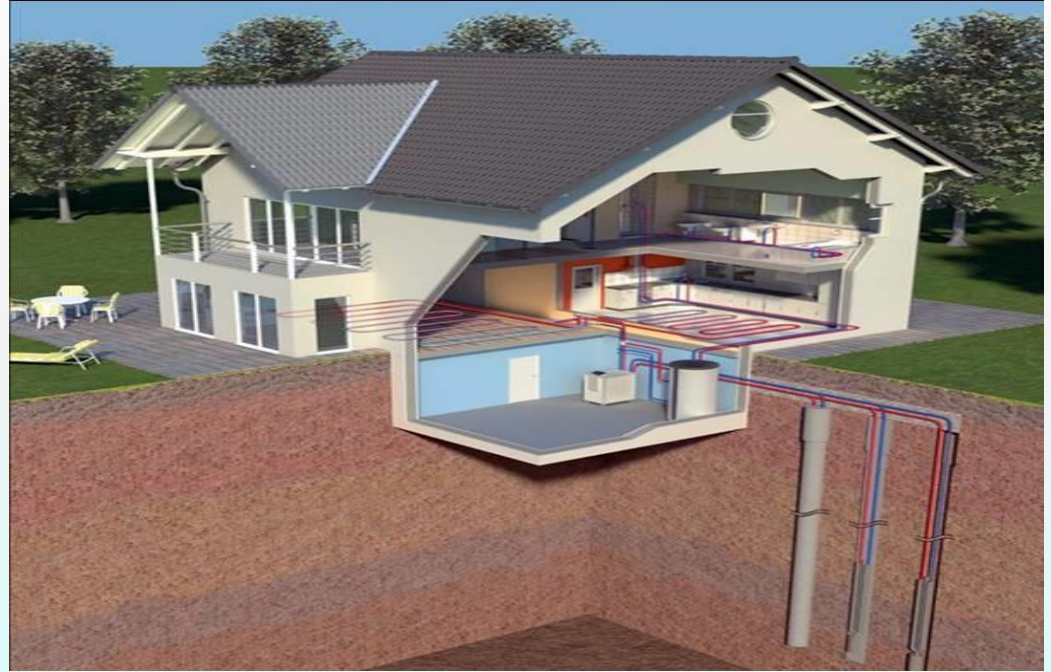
A typical model of geothermal heating using shallow geothermal resources and a heat pump system
