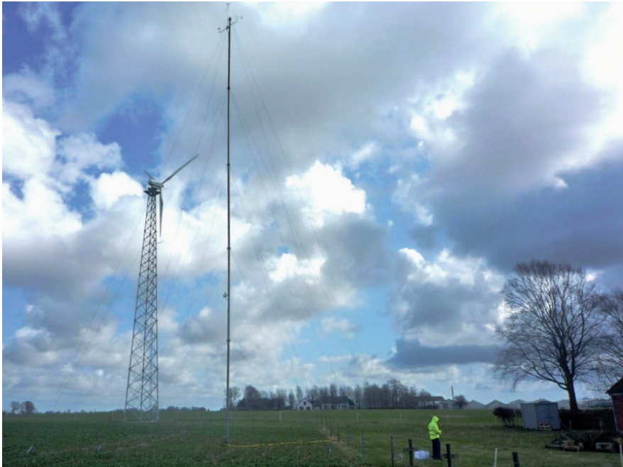
Figure 11: A WindEn 45 turbine undergoes testing by Intertek
