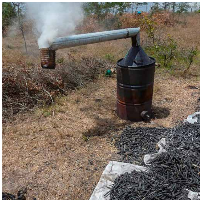
Improved Kinyanjui "Green Cap" barrel kilns Photograph: Cookswell Jikos
