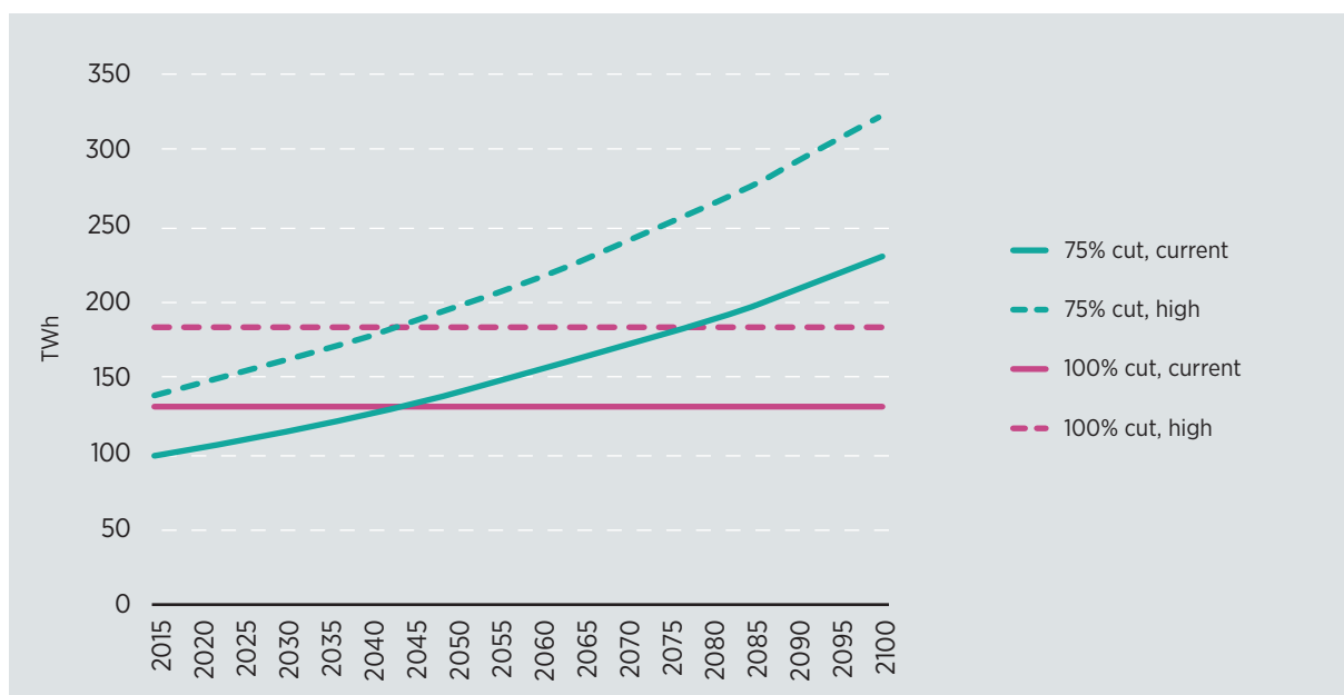
Figure 5.3 Primary energy from forests with different harvest rates and wood use
