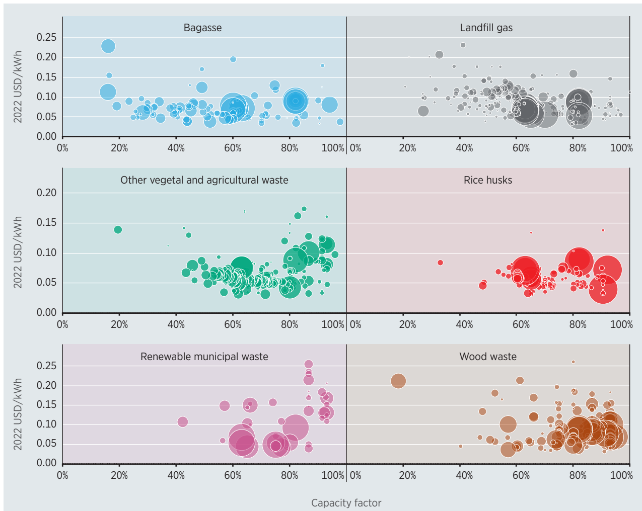
Figure 8.6 LCOE and capacity factor by project of selected feedstocks for bioenergy power generation projects, 2000-2022
