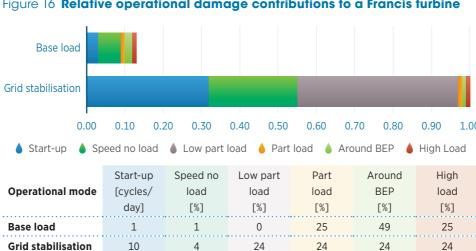
Figure 16 Relative operational damage contributions to a Francis turbine
