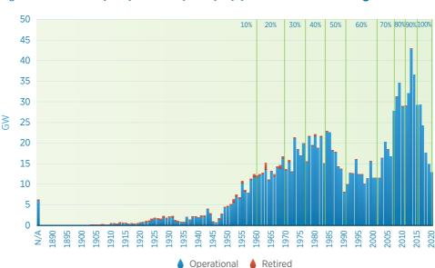
Figure 11 Global hydropower capacity by year of commissioning
