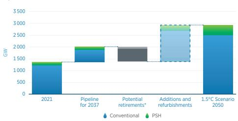
Figure 13 Necessary hydropower capacity additions by 2050
