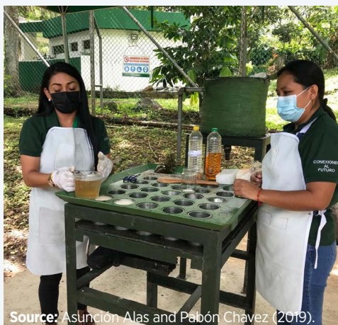
Photograph 7 LaGeo-FundaGeo's geothermal heat use prototypes for melting wax for candle making and honey processing in El Salvador
