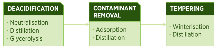
Figure 20 Pretreatment of oils to optimise the yield of biodiesel through transesterification
