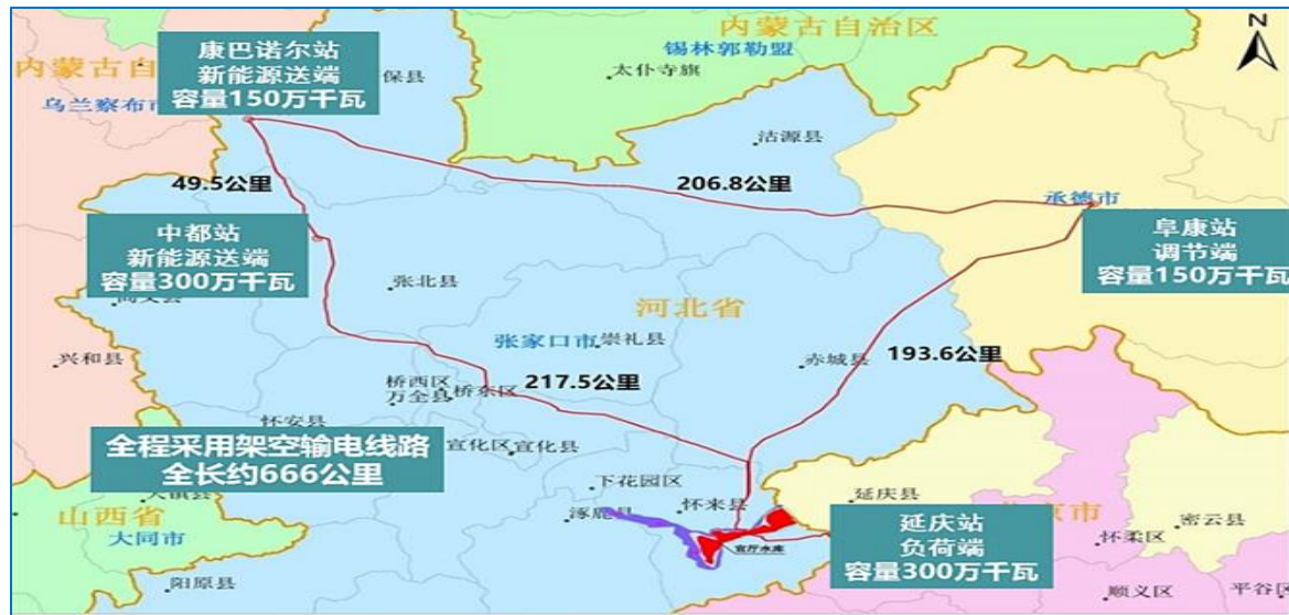
Zhangbei four-terminal VSC-HVDC power grid wiring diagram
