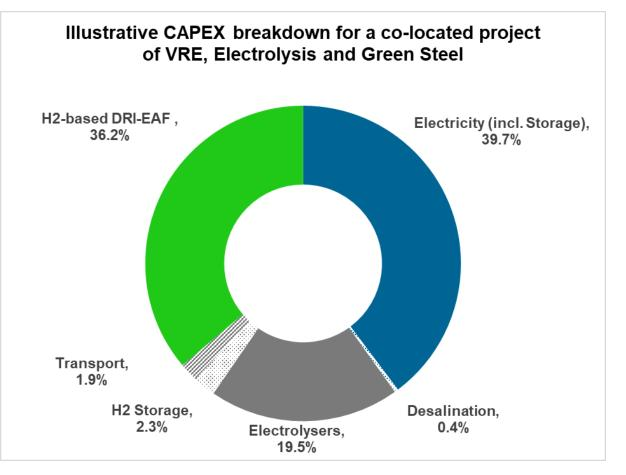
Illustrative calculation based on 50% solar and 50% onshore wind in a favourable location (LCOE USD 30/MWh), USD 550/kW electrolyser costs, 50% capacity utilisation rate for the electrolyser, and availability of geological storage for  $H_2$ .
