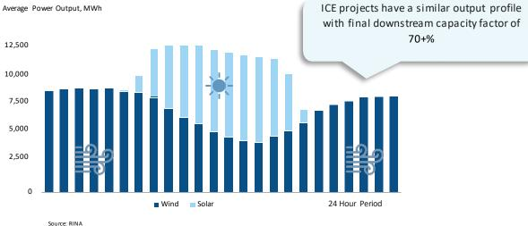
Complementary Wind / Solar Output Drives Maximum Capacity Factor
