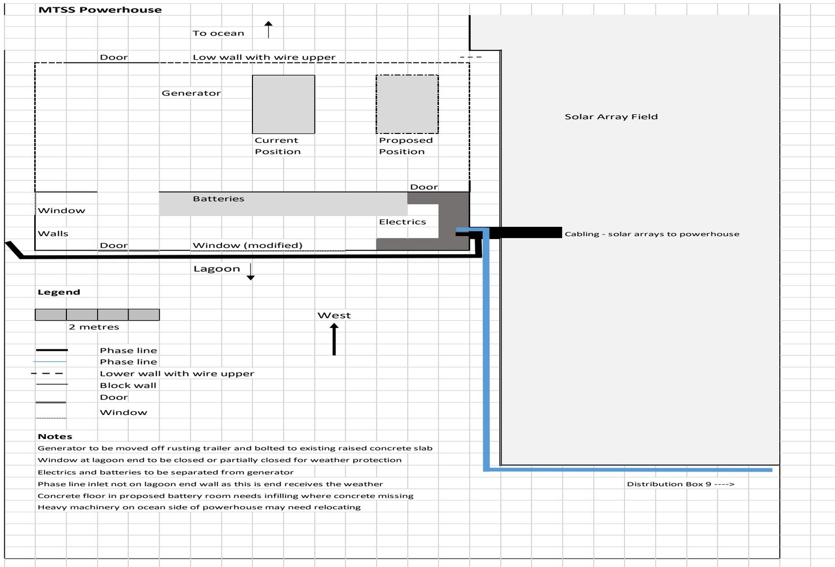
Figure 13. MTSS Powerhouse Schematic diagram including proposed solar pave array field
